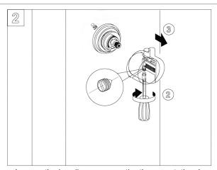
Loosen the handle screws on the ther mostatic mixer knob (rotate the screws 2 to 3 rotations).
