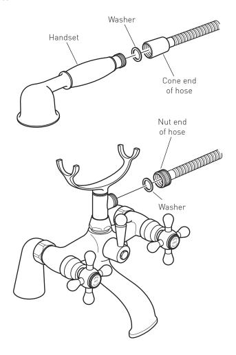
Place one of the rubber washers into the cone end of the hose and screw to the handset.
