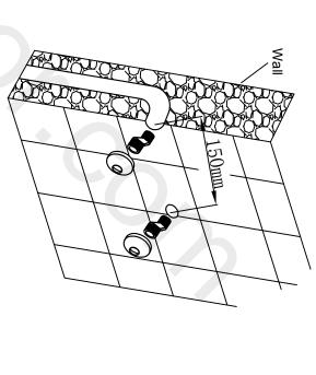
2. Fix the connector of shower valve to the off-set connector with spanner. Please use a cotton sheet inside of spanner in case on right, otherwise it will affect the performance. of any scratches. Make sure hot inlet on the left and cold inlet
