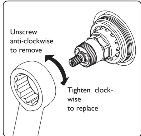
3. Remove the piston and thermostat assembly and place into a bowl.
