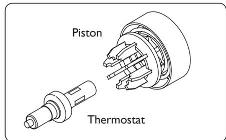
4. Grease the seals with a silicon grease and carefully refit.
