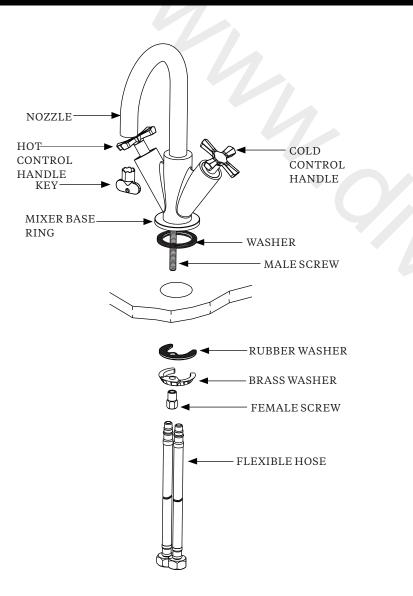
First shut off your water heating system, then with your mains stop cock closed, open the lowest cold and hot taps in the house and allow to run until the cold storage tank and pipes are empty (the hot storage cylinder always remains full). Fitting isolating value to inlet feeds is recommended for ease of maintenance.
