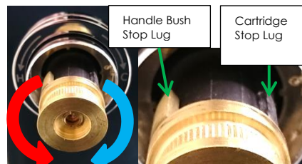
5. Now re-fit the Handle Bush so that the Stop Lug is not in contact with the Cartridge Stop Lug and rotate the Handle Bush fully clockwise until a 'click' is heard. Should the Stop Lugs come into contact before the click, simply remove the Handle Bush, turn it half a turn anti-clockwise, fit it back onto the cartridge and continue to rotate it clockwise. Repeat this process until you hear the click.
