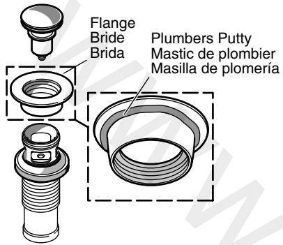
**2** Insert the assembly. Attach the flange.
