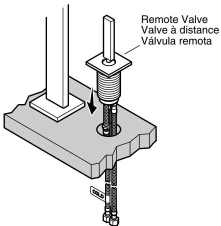
**8** Position the remote valve with the cold water supply on the left and the spout outlet connection toward the front of the sink.
