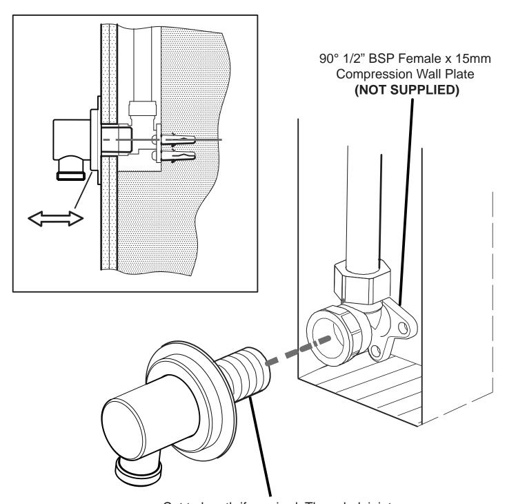
Cut to length if required. Threaded joint connections should be made with PTFE tape. Oil based, non setting jointing compounds should not be used.
