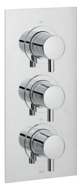
**DESCRIPTION:** DX Celsius concealed 2 outlet, 3 handle thermostatic shower valve wall mounted with rectangular backplate thermostatic cartridge V-001C-PLA flow cartridge C-301-RTC 2 x 3/4" female inlets 2 x 3/4" female outlets includes 3/4" - 1/2" adaptors inc. bleed valve for system flush on installation min-max wall mount 70-95mm optimum installation depth 82mm minimum operating pressure 0.2 bar LP (shower) minimum operating pressure 1.0 bar MP (bath)
