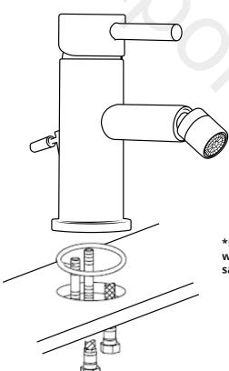
\*Remember to install the 'O' ring or washer between the mixer body & sanitary ware\*
