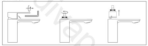
Remove the push cover. Using an Allen key loosen the grub screw this will allow the handle to be removed. Unwind the shroud, Care-fully with a spanner loosen the locking nut, this will allow the cartridge to be taken out and replaced. When inserting the new cartridge make sure the 2 locating points align, then re-assemble.
