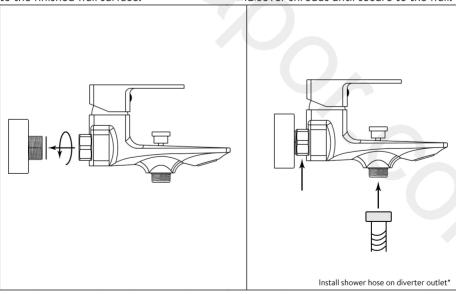
Install the washers/filters in to the mixer body, then hand tighten the mixer to the eccentrics, ensure level-ness. Place a cloth over the nuts to protect from scratching when fully tightening with a spanner. Turn on the water and test.
