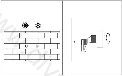
Pre-Install two ½" female fittings, level and 150mm apart, these fitting must be flush to the finished wall surface.
