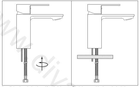
Install the threaded rods and hand-tighten the flexi-pipes into the bottom of the mixer in the basin/countertop. body.
