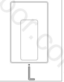
Install the handle onto the cartridge pin and secure by tightening the grub screw. turn on the water and test the mixer.
