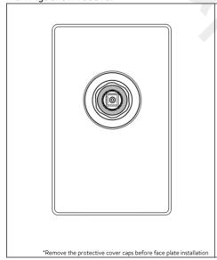
Apply the surrounding finishes, fit the face-plate onto the valve body.
