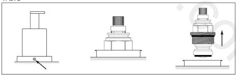
Remove the grub screw on the reverse side of the valve body and lift up. Using a spanner carefully unwind the cartridge from the valve housing. Remove, replace and re-assemble.
