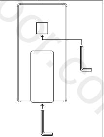
Install the diverter knob and mixer handle, secure by tightening the grub screws.
