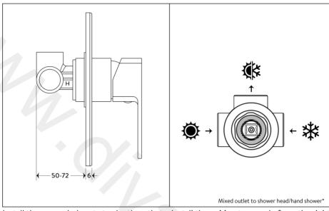
Install the concealed part at a depth so that finished surface is between the Min/Max markings shown above.
