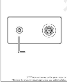
Apply the surrounding finishes, fit the face-plate onto the valve body and secure by installing the spout connector.
