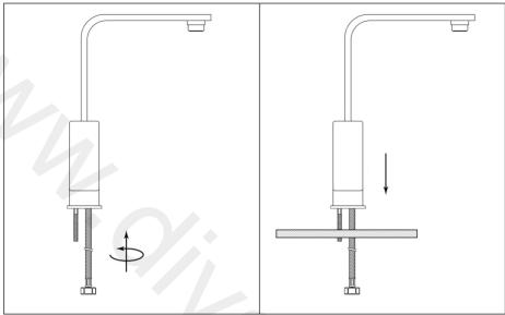
Install the threaded rods and **hand**-tighten the flexi-pipes into the bottom of the mixer
