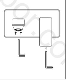
Install the spout and handle, secure by tightening the grub screws. Turn on the water and test the mixer.
