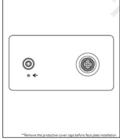
Apply the surrounding finishes, fit the face-plate onto the valve body and secure by installing the face plate screw.
