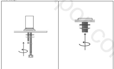
Slide the rubber 'C' washer followed by the metal 'C' washer and tighten the back nuts with a spanner to secure the mixer valve.
