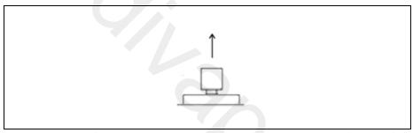
All diverters only function when the main water supply is turned on, for deck/floor mounted bath/shower mixers pull the diverter knob.
