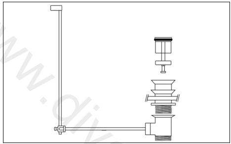
Install the waste ensuring that the foam washer is in between the waste and the basin on the top portion of the waste, the rubber washer is to be placed under the basin before the bottom part of the waste is connected and tightened up.
