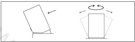
To control water flow on deck mounted mixers push the handle backward. To adjust the temperature, turn the handle and tilt to the right for cold water and left for hot water.
