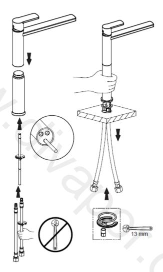
Place the threaded rod and 2 flexible pipes into the body of the mixer, place the assembly over the extension piece and through the basin / counter, From the underside, place the 'O' ring followed by the metal 'C' washer onto the threaded rod, then tighten to clamp the mixer to the basin / counter with the back nut, being careful not to over tighten.
