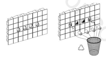
Apply the surrounding finishes, once the surrounding finishes have been applied (Tiles/Marble etc.) remove the protection covers and the metal plates and discard.
