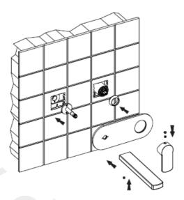
Install the spout extension and secure with the bolts provided. Screw on the cover shroud to the mixer body.
