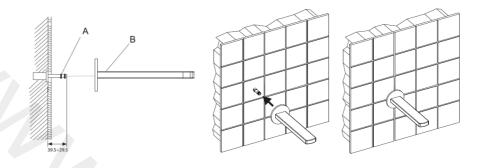
Install the spout connector (A) at the depth advised on the diagram above. Push the spout onto the connector and secure with the grub screw on the underside.
