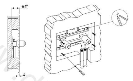
Install the mixer housing (1) at a depth so that the finished surface is between the Min/Max distance markings shown in the diagram. Mark the holes on the fixing bracket. Drill and plug these before fixing the bracket. Connect the Hot and Cold water supplies to the mixer and cap off the outlet connection, pressure test to check for leaks at the connections.
