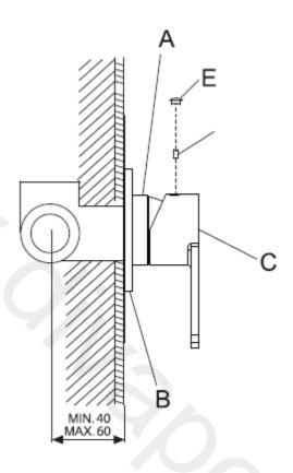
Install the mixer housing (A) at a depth so that the finished surface is between the Min/Max distance markings shown in the diagram.
