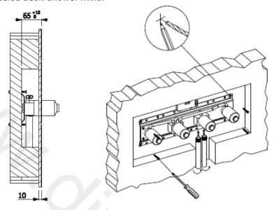
Install the mixer housing (1) at a depth so that the finished surface is between the Min/Max distance markings shown in the diagram. Mark the holes on the fixing bracket. Drill and plug these before fixing the bracket. Connect the Hot and Cold water supplies to the mixer and cap off the outlet connection, Connect the Hot and Cold water supplies to the mixer and pressure test to check for leaks at the connections.
