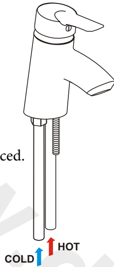
Figure 2 Bath Filler Connections
