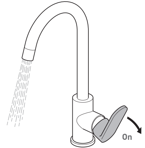
Pulling the mixer lever away from the tap body will increase the flow of water.
