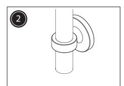
Slide the rigid riser rail through both wall brackets.
