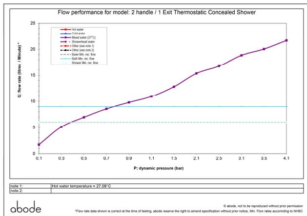
• **Min / Max water pressure (bar):** 0.40\* / 5.00
