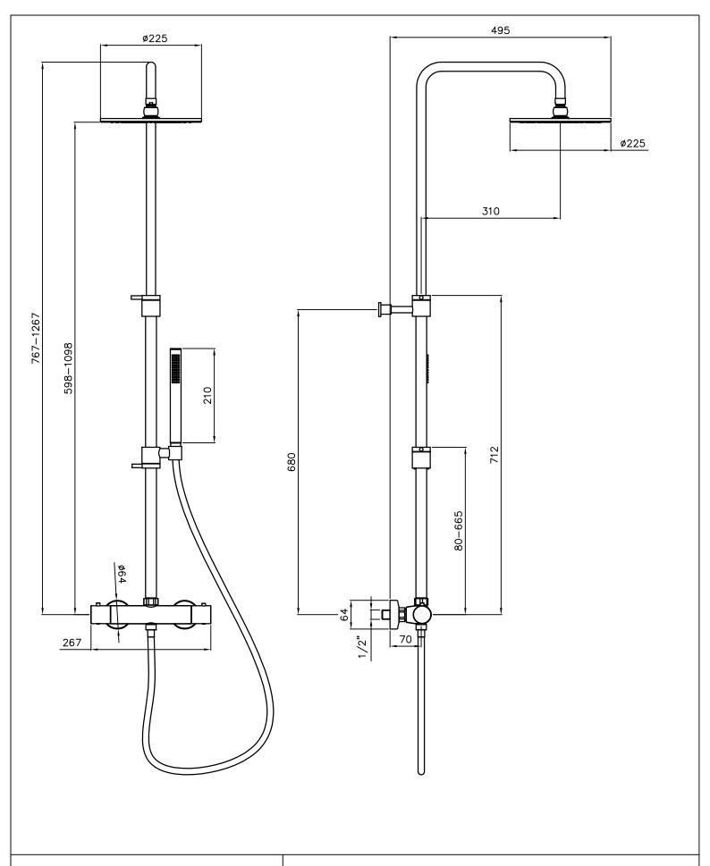
Circular Wall Mounted thermostatic valve with rigid riser, fixed head and shower kit AB4190 v1
