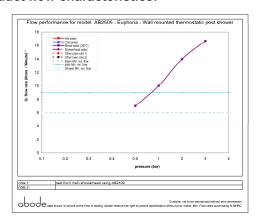
Min / Max water pressure: 1.25 / 5 bar
