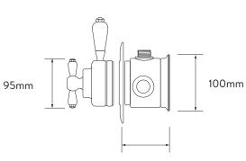
Distance from back of valve to finished wall surface (includes 10mm allowance for tiles) Min. 68mm Max. 82mm
