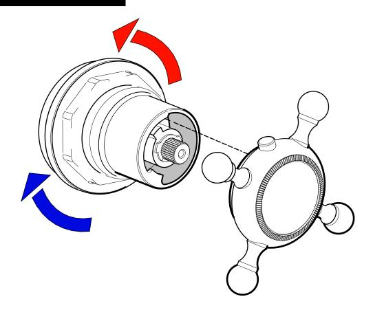
Using the control knob rotate the thermostatic spindle anticlockwise to set the maximum hot water temperature. The recommended maximum should not exceed **41°C**. Then line up the screw head on the back of the control knob with the first stop on the stop ring, push the control knob onto the spline and tighten the grubscrew. The temperature override button can be used to increase the temperature for bath fill installations.
