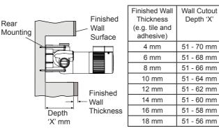
With the outlet port facing up place the Mixer Valve square central and level in the hole, mark the positions of the fixings holes on the wall. Using a minimum of 2 screws (supplied), screw the mixer valve to the wooden noggin
