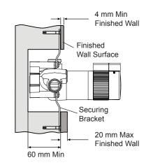
Fit the securing brackets to the mixer with the bracket securing screws. Important! Make sure that the correct holes are used Note! The securing brackets can be rotated for suitable fixing points
