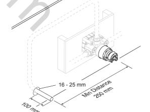
Fit the compression nuts and olives onto the pipework, connect the pipes and tighten the compression nuts. Important! Make sure that the outlet pipework protrudes through a Ø16 - 25 mm hole in the wall or stud partition by approximately 100 mm and temporarily cap off.
